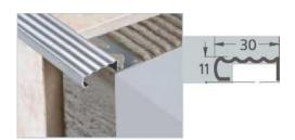
The profile is designed to protect and to decorate edge of step encased by ceramic tile. Special shape and material of production allows using it at the highest foot traffic. Invisible fixing on glue for tile.
