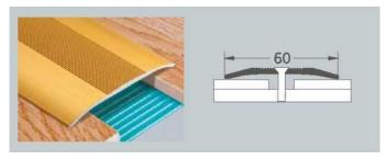
New form of the profile allows you to use it with level difference of floor coverings up to 5 mm. Suitable for all types of floor coverings. Visible fixing - dowel/screw.
